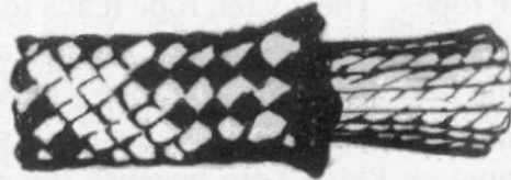
Static, kernmantle rope showing core (kern) and sheath (mantle).
