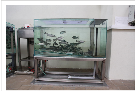
Drinking water pollution detector Rainbow trout ( Oncorhynchus mykiss ) are being used in water purification plants to detect acute water pollution
