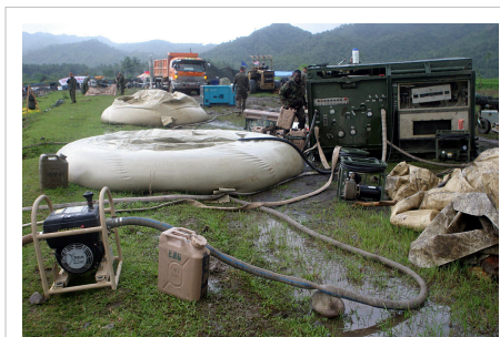
Marines from Combat Logistics Battalion 31 operate ROWPUs for relief efforts after the 2006 Southern Leyte mudslide
