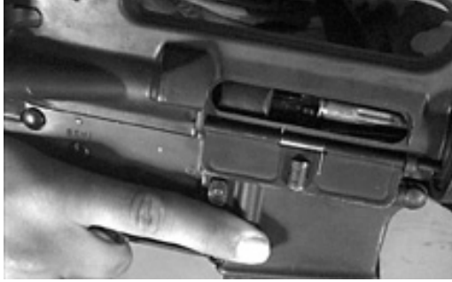
Figure 3-15. Brass Obstructing the Chamber.
